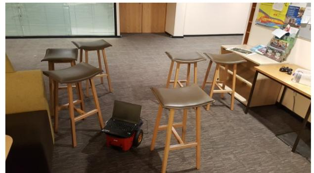
Fig. 9. Actual layout of obstacles (stools) used for local obstacle avoidance test. Robot included for scale
