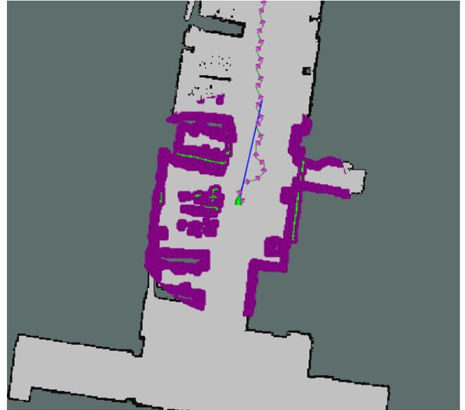
Fig. 5. Global Path (purple arrows) shown before dynamic obstacle. Green pointer shows the robot's position. Blue line is drawn to the current goal position.
